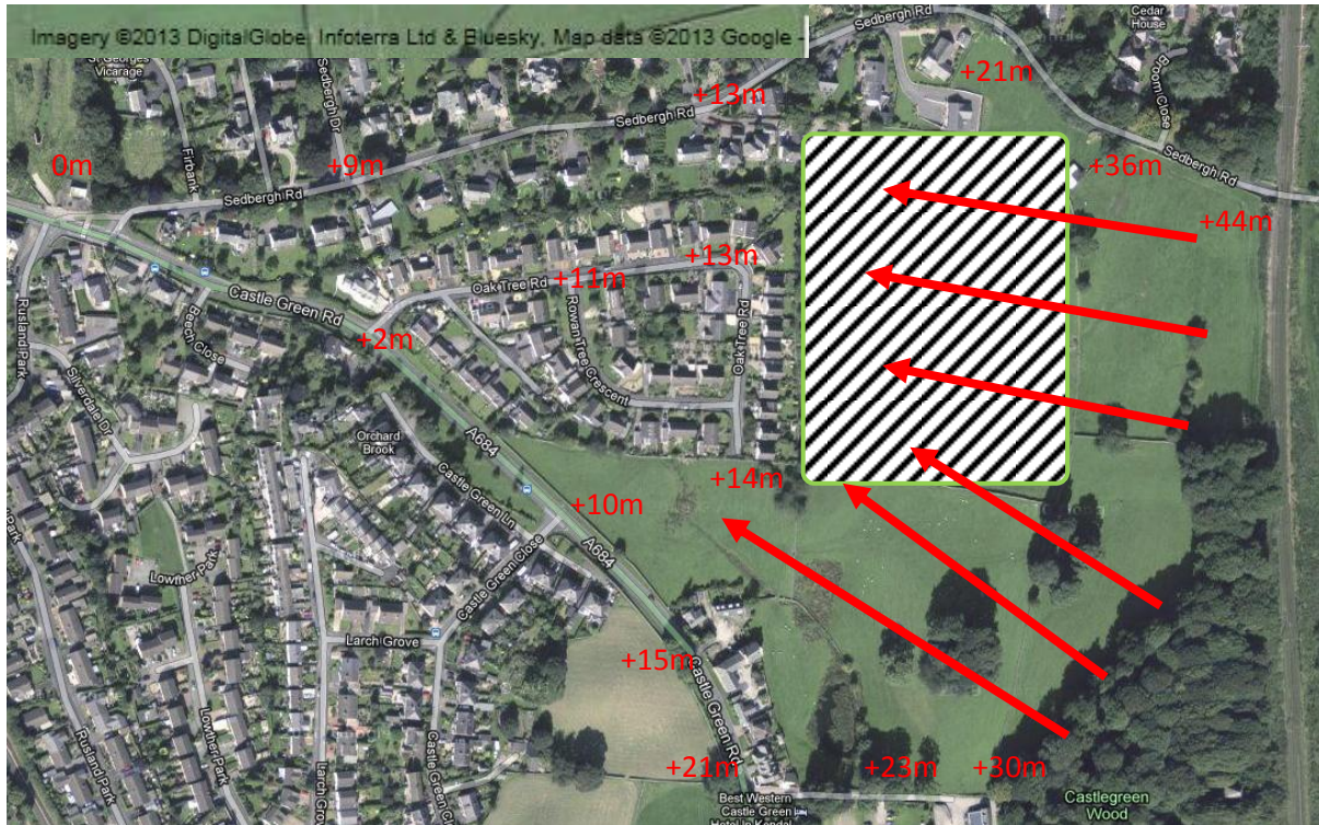
Figure 2.4 – Topographic data and probable flood flow paths
